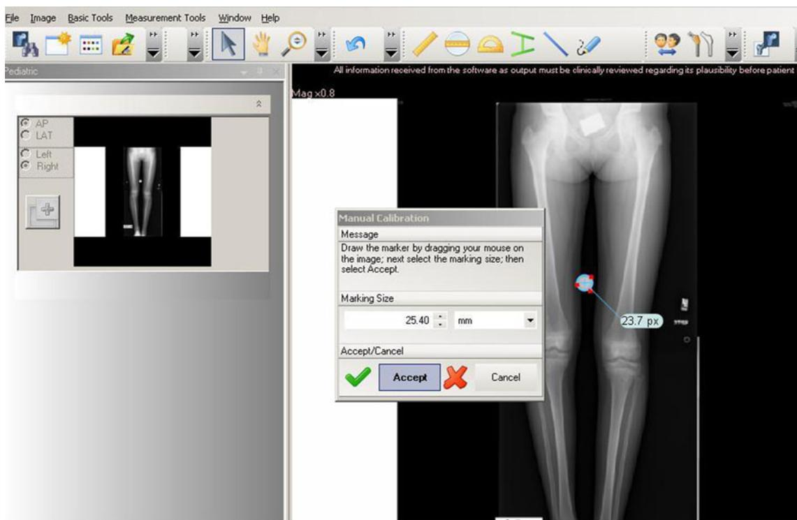
Fig. 6 Standing view radiograph of a leg length discrepancy (LLD) patient; calibration with the metal ball
